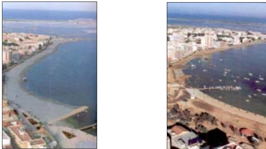
Figs. 37 & 38: Before and after views of beach nourishment in San Pedro del Pinatar (MOPT, 1993).
